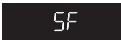
Figure 28: Display showing Sabbath failure
