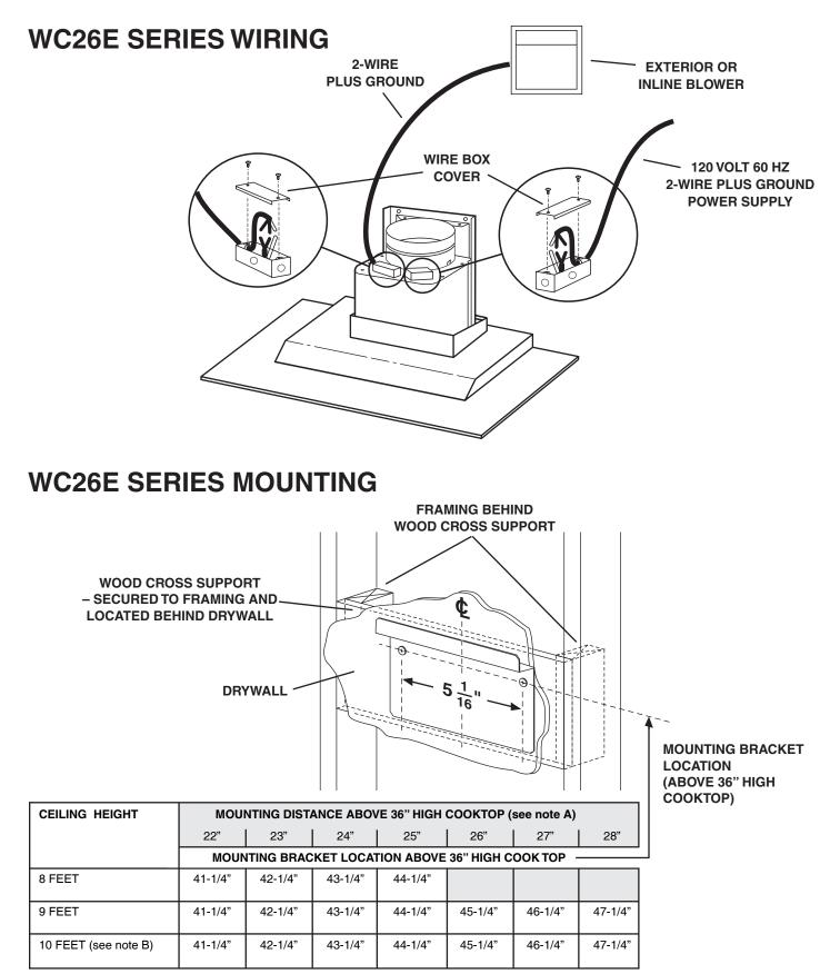
A. Minimum hood distance above cooktop must not be less than 22". A maximum of 28" above the cooktop is highly recommended for best capture of cooking impurities. Distances over 28" above the cooktop are at the installer's and user's discretion - providing that ceiling height and flue length permit.
