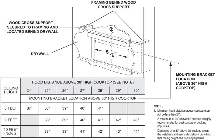
Requires optional 10-foot flue extension model RFX5304 (ducted) or RFXN5304 (nonducted).
