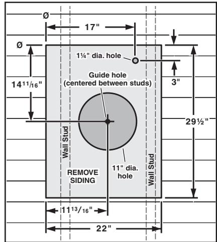
3. From the outside, use the guide hole as a starting point to lay out the installation:
