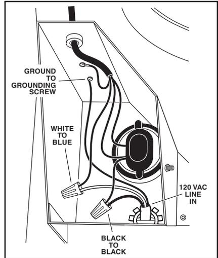
being used. Connect black to black, white to blue, and green or bare wire to grounding screw.
