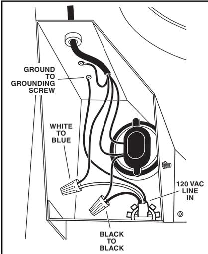
proper connector for the type of wiring being used. Connect black to black, white to blue, and the green or bare wire to grounding screw.
