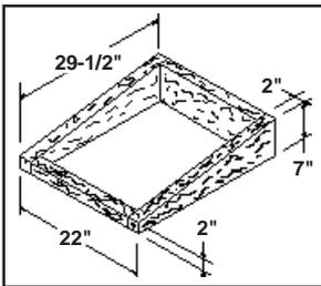
4. For flat roof installations, build a curb that will
