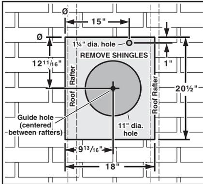
3. From the outside, use the guide hole as a starting point to lay out the installation:
