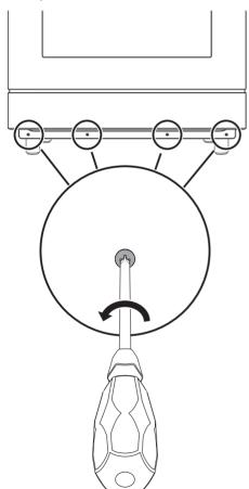
2. Position the front skirting at the bottom of the appliance and line up the holes of the front skirting with the holes on the base of the appliance.
