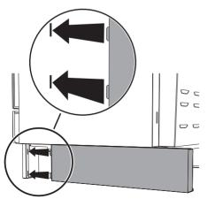
4. Line up the hole on the side skirting with the rear hole on the base of the appliance.
