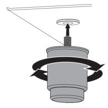
The appliance must sit level on the floor to ensure stability.
