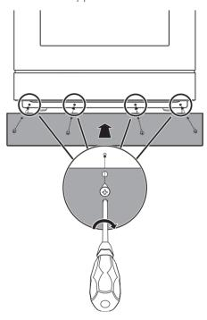
3. Fasten the front skirting to the appliance using the previously removed screws.
