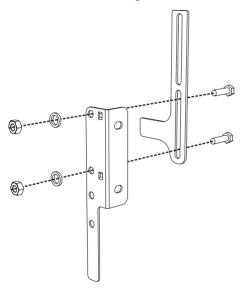
2. Align the base of the hook on the fastening bracket with the base of the slot on the wall fastening plate.
