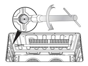
**5) WARNING:** The tightening torque of the nozzle must be equal to 4 Nm - 14.4 Ozf.
