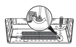
5) Remove the burner from its place by sliding it out and moving it to the side. (Make sure not to damage the thermocouple or the spark electrode during this operation).
