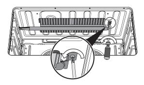
3) Remove the burner by sliding it from its place and reposition it as shown in the picture. (Make sure not to damage the thermocouples and the spark electrode).
