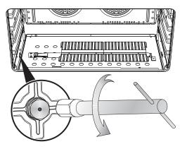
**7) WARNING**: The tightening torque of the nozzle must be equal to 4 Nm.
