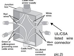
Connect to a 20A fuse or circuit breaker. Connect to copper wire, or, if connection is made to aluminum house wiring, use UL-listed or CSA-approved connectors that are approved for joining aluminum and copper wires.
