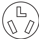
3-wire receptacle (10-30R)
