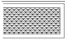
For best performance: Replace grease filters with half-moon openings facing out - and in orientation shown.
