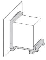
A frame should be constructed 2" (51 mm) setback from the front face of the product to both push the product up against and conceal the cutout clearance around the front frame.
