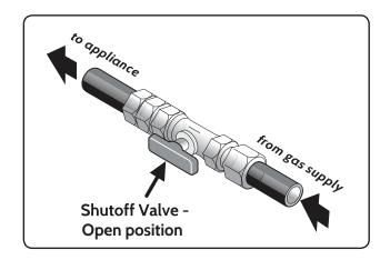
7 Check for gas system leaks with a manometer. If a manometer is not available, test all connections by using the supplied leak detection solution.
