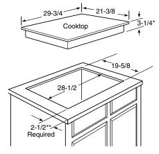
\*Depth of unit at conduit connection location (rear) is 6-1/2" on models PP980/950 and 4-5/8" on models PP975/972/962/945/942/932/912, JP655/356/346.
