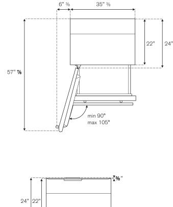
INSTALLATION: There shall be a space not less than 1 inch from the top of your refrigerator, not less than 1/4 inch from both sides and 1 inch or more from the back of the refrigerartor to the adjacent walls respectively. This requirements is good for open and close of the door and also for heat emission.
