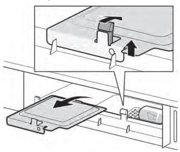
2. Remove old light bulb and replace only with equivalent 30 watt bulb available from parts distributor. Bulbs are also available at most hardware stores or lighting centers.
