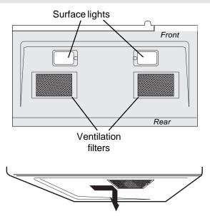
1. To remove the exhaust ventilation filters, slide the filter to the rear. Then pull filter downward and push to the other side. The filter will drop out. Repeat for the 2nd filter.
