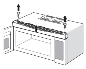
4.Remove the charcoal filter by pushing it inwards, then turn and pull it away from the unit.
