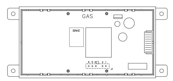
2. (F30 or F31) Check resistance at room temperature, if less than 500 ohms, replace RTD Sensor Probe. Check for shorted Sensor Probe harness between EOC & Probe connector.
