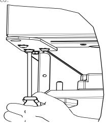
Note: When reversing the door, it is necessary to remove and switch the shelf-mounting hardware. This will allow the shelf to extend out of the unit beyond the door.
