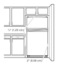
To ensure proper ventilation for your convertible refrigerator/freezer, allow for ½" (1.25 cm) space on each side and at the top. When installing your convertible refrigerator/freezer next to a fixed wall, leave 2" (5.08 cm) minimum clearance on each side to allow for the door to swing open.
