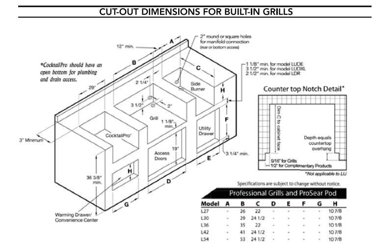
Note: Insulated jacket required for all grills installed into a combustible enclosure. See detail below.
