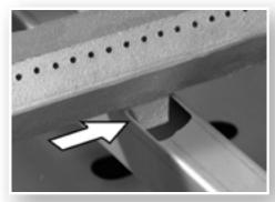
The main burners must sit level and firmly on the frame with their mount-ing legs inserted into the frame slots.
