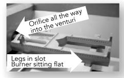
3) Then pull to the rear of the grill so the burner head comes off the brass orifice at the front.
