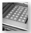
Flip the trays over and put them back in place over the burner. Light the burners and set them to "HI" for 5 - 10 minutes
