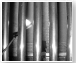
Push and turn the corresponding burner control knob to "LITE". If the burner doesn't light within 5 seconds turn the knob off and wait 5 minutes before attempting to light it again.
