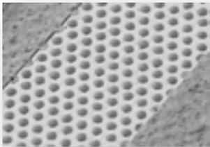
These holes focus the flame on the surface of the
