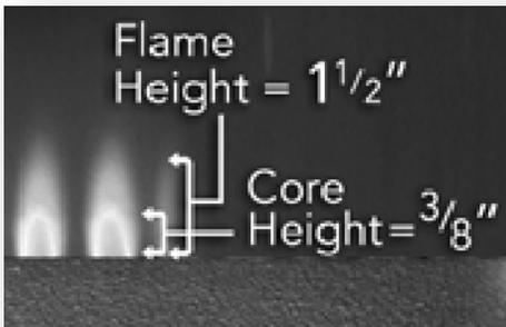
Flames should be blue and stable with slight yellow tips. The bright-blue core should be about 3/8 inch high with a total flame height of about 1
