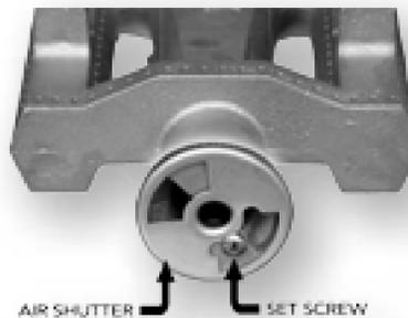
If the flame is excessively yellow, indicating insufficient air, CAREFULLY turn the air shutter counter-clockwise to allow more air to the burner.
