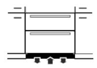
It is important to use the provided cover grille for the ventilation opening. This opening must not be covered with a cabinet base.
