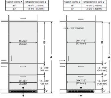
The height of this panel can be reduced by up to 2" to accommodate higher toe kicks
