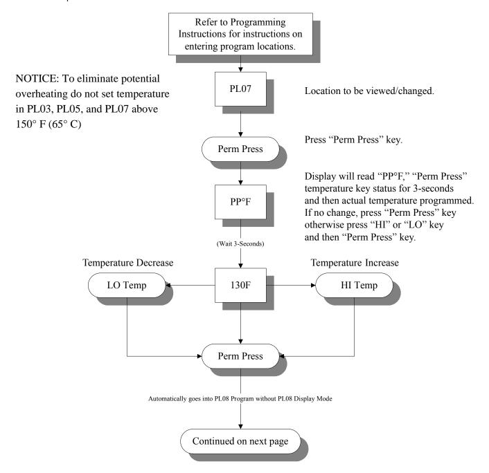
Summary: Perm Press Temp is programmable from a minimum of 100 °F to a maximum of 190 °F in ten-degree increments or from a minimum of 38 °C to a maximum of 88 °C in five-degree increments.
