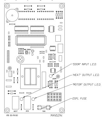
There are three L.E.D. indicators ("red" lights) located at the lower back side area of the microprocessor controller (computer) which are identified/labeled as "DOOR," "HEAT," and "MTR" (motor). These L.E.D.s indicate that the output s of the microprocessor controller (computer), or in the case of the door switch, the inputs are functioning.
