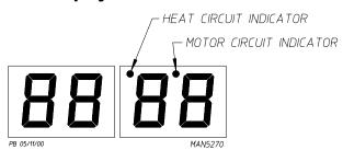
The L.E.D. indicator dot s located at the top portion of the display indicates the various microprocessor controller (computer) output functions while a cycle is in progress. These dots do not necessarily mean that the outputs are functioning. They are only indicating that the function (output) should be active (on).
