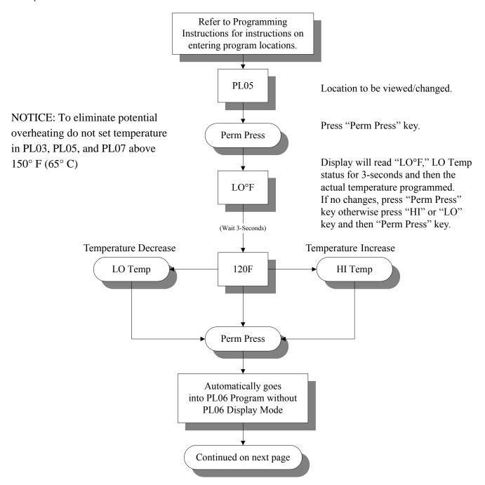
Summary: LO Temp is programmable from a minimum of 100 ° F to a maximum of 190 ° F in ten-degree increment s or from a minimum of 38° C to a maximum of 88° C in five-degree increments.
