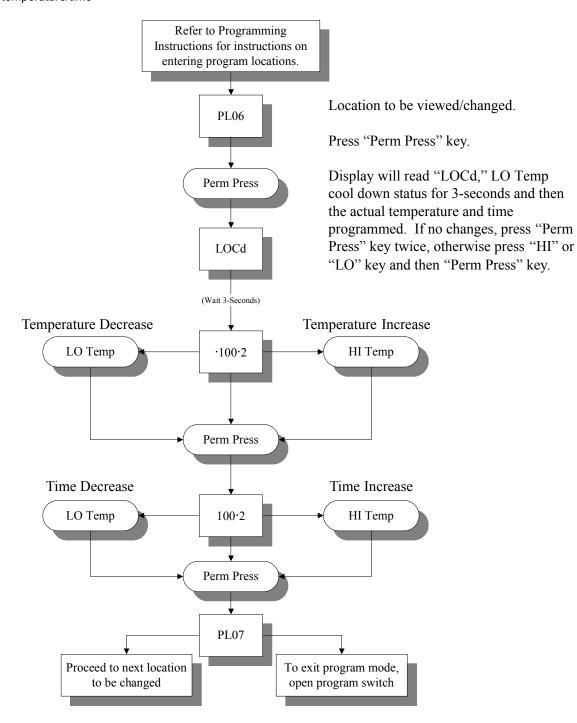
Summary: Cool down temperature is programmable from a minimum of 70° F to a maximum of 190° F in ten degree increments or from a minimum of 21° C to a maximum of 88° C in five-degree increments.
