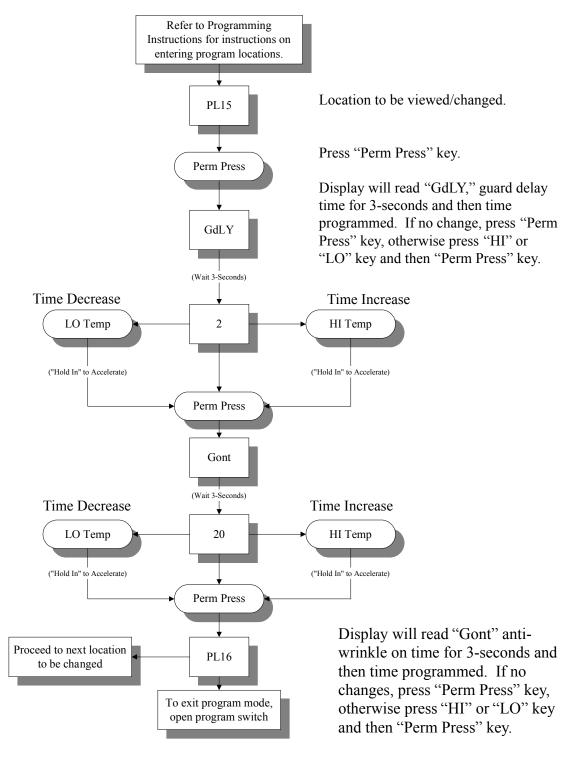
Summary: Guard delay time is programmable from 1 to 9 minutes. Guard on time is programmable from 1 to 99-seconds.
