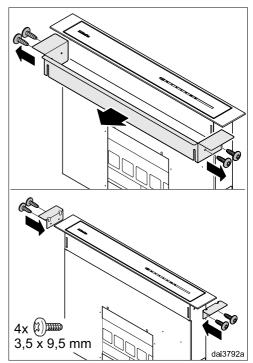
Unscrew the screws on either side, remove the support bracket and replace it with the two small angle brackets supplied.
