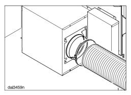
Secure the exhaust ducting to the exhaust socket, e.g., with a hose clip (available as an optional accessory) on flexible ducting.
