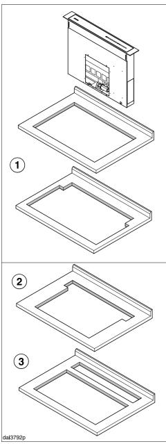
A support bracket is mounted on the downdraft. It serves as a support for the cooktop when the downdraft extractor and the cooktop are installed in a common cutout ①. In the following situations, the support bracket should be replaced with two small angle brackets:
