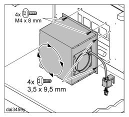
Rotate the motor so that the exhaust connection points in the required direction and secure it to the downdraft.
