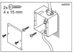
Secure the connection box to a suitable place, e.g. a cabinet wall.
