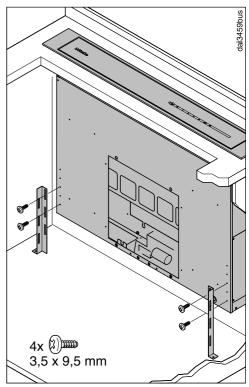
Secure each of the lower brackets with two screws on the casing, so that the feet rest on the floor of the housing unit. To do this, you can also rotate the brackets when fitting them.
