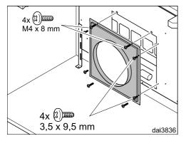
If an external blower is being used, the appropriate vent connector is fitted instead.
