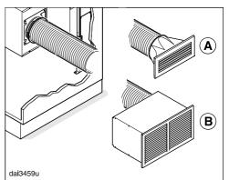
connect a DUU 151 recirculation conversion kit (A) to the exhaust socket. The downdraft grease filters must be fitted with DKF 22-1 charcoal filters (see "Cleaning and care")
