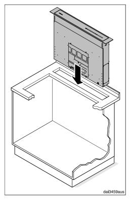
Place the downdraft carefully into the prepared cutout (see "Appliance dimensions").
