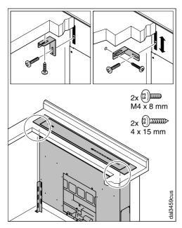
Fit the upper brackets loosely to the downdraft casing.
