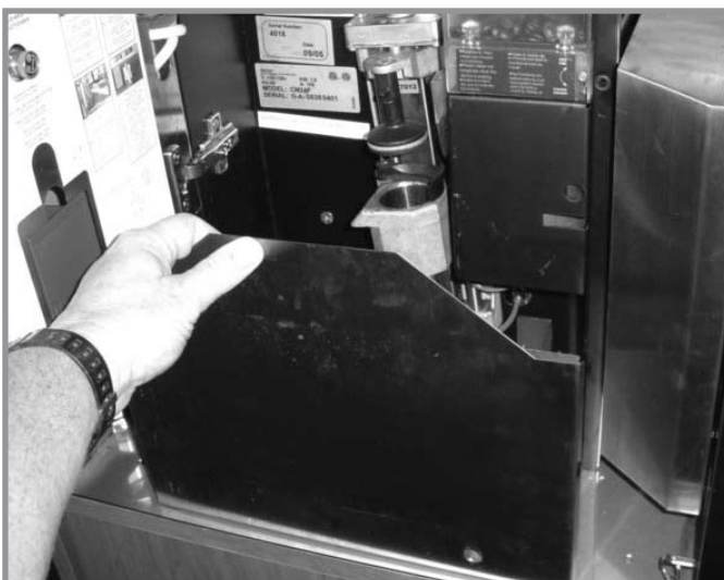
Used Coffee Grounds Bin Removal
