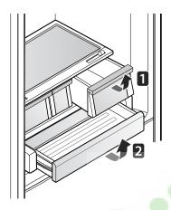
To install, slightly tilt up the front, insert the drawer into the frame and push it back into place.
