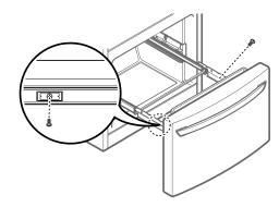
4 With both hands, grip both sides of the drawer and pull it up to remove it from the rails.
