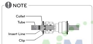
1) Gently press the Collet and insert the tube until only one line shows on the tube.
