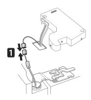
4 Make sure that the door-switch located inside the cover is tightly connected. Position the cover in its place. Insert and tighten the cover screw 2.
