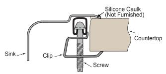
3-1/2" (89mm) (192mm) Sink with Drain Kit Installed
